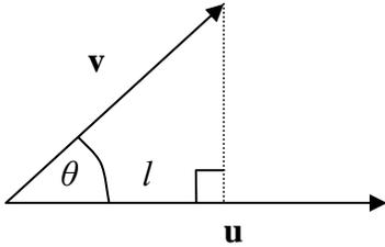
The relation  $\mathbf{u} \cdot \mathbf{v} = \|\mathbf{u}\| \|\mathbf{v}\| \cos \theta$  can also be used to provide a simple way of calculating the **scalar projection** of one vector in the direction of another. If we let  $l$  denote the orthogonal (perpendicular) projection of  $\mathbf{v}$  in the direction of another vector  $\mathbf{u}$ , then from the diagram we see that  $l = \|\mathbf{v}\| \cos \theta$ . We can solve for this in the previous relation to get:
