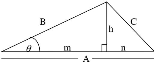
$$\begin{aligned} B^2 &= m^2 + h^2 \quad \text{and} \quad C^2 = h^2 + n^2 \\ A &= m + n, \text{ so we can write } n = A - m. \\ \text{If we substitute this, we get:} \\ C^2 &= h^2 + (A - m)^2 = h^2 + A^2 - 2Am + m^2 \\ &= B^2 + A^2 - 2A(B \cos \theta) \\ &= A^2 + B^2 - 2AB \cos \theta \end{aligned}$$
