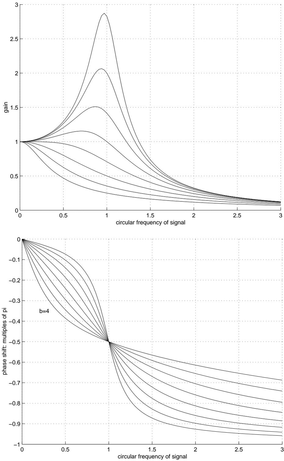
FIGURE 8. Second order amplitude response curves
