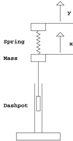
FIGURE 6. Spring-driven system
