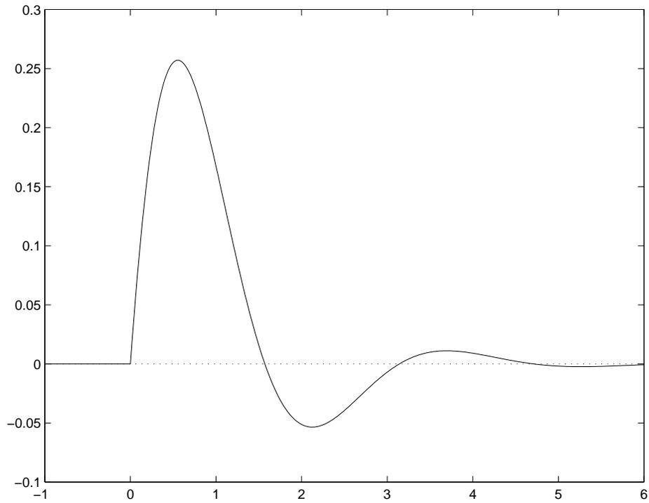
FIGURE 13. The weight function for  $\ddot{x} + 2\dot{x} + 5x$
