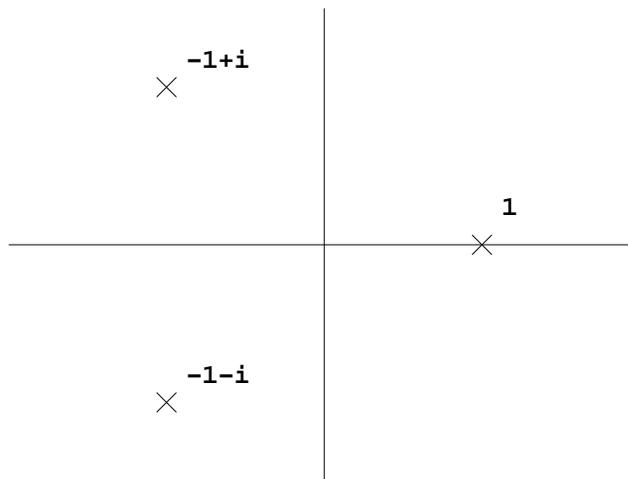
FIGURE 15. Pole diagram for  $1/(s^3 + s^2 - 2)$
