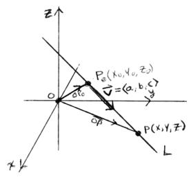
This construction can be done in any dimension, including  $\mathbf{R}^2$ . In this case, the parametric equations become simply  $\begin{cases} x = x_0 + at \\ y = y_0 + bt \end{cases}$ . Note that with direction vector  $\mathbf{v} = \langle a, b \rangle$ , the slope of the line would be  $m = \frac{b}{a}$  (if  $a \neq 0$ ) and we can solve for the common parameter to get  $t = \frac{x - x_0}{a} = \frac{y - y_0}{b}$ . This is known as the symmetric equation for the line (assuming neither a)
