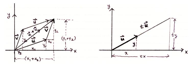
The left diagram illustrations why the algebraic definition for vector addition corresponds to "tip-to-tail" addition of the respective vectors when thought of as (equivalence classes of) directed line segments. This is also known as the **Parallelogram Rule** because this **resultant vector** is realized by following consecutive edges of the parallelogram whose parallel sides are determined by the respective vectors.
